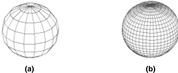
Figure 1: A simple example illustrating two levels of detail of a polygon sphere. Figure 1(a) contains 112 polygons, and Figure 1(b) contains 1104 polygons.
